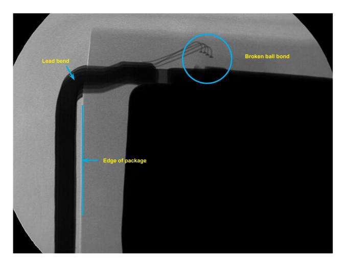
Figure A-3. This x-ray image shows a side view of a package with excessively close lead-bending to the package body. No clamping of the leads was used. The result was that the wire ball bond was broken due to physical trauma upon the lead due to the bend without clamping.
