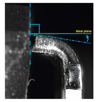
Figure 27. This is an example of an acceptable pin bend, where clamping above and below the pin was used. Ideally, there should be no deflection of the pin from the perpendicular, however, a slight amount may be acceptable.
