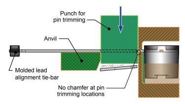
Figure 15. Clamping solution for pin 3 trimming; clamps form an anvil on the package case side of the punch, with a second anvil on the outside
