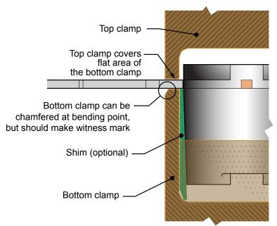
Figure 12. Close-up view of clamping solution; note that, if pins are to be trimmed rather than bent, there should be no chamfer under those pins, and a sharp 90-degree edge should be present instead (see figure 10)
