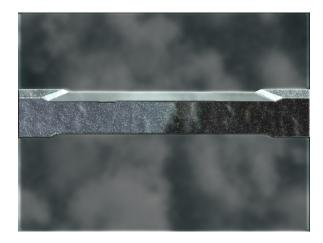
Figure 6. Maximum acceptable embossment that would result from a proper clamping. Dual shiny parallel bands should uniformly extend across the pin on both sides.
