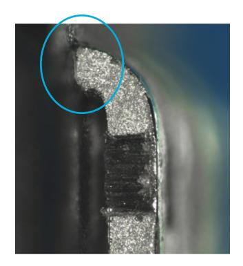
Figure 28. This is an example of an unacceptable pin bend, showing no clamping was used and the pin too close to the package case. Circled area of disturbance indicates potential internal damage.
