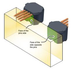
Figure 4. Flat sides are designed into the Allegro back-biased products to allow reliable orientation with minimal contact.
