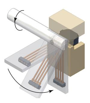
Figure 16. Paddle forming fixture; clamping above and below the pins is required to prevent damage to the device
