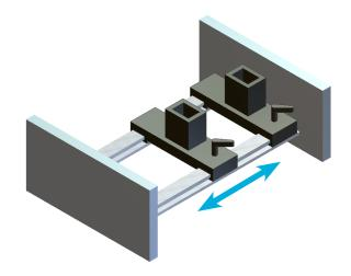
Figure 7. Commercial linear bearing mechanisms can be used for swapping tools in-line.
