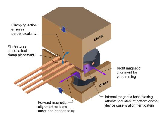
Figure 13. Illustration of effective use of the inherent magnetic qualities of the device to assist in mounting and alignment in the clamp
