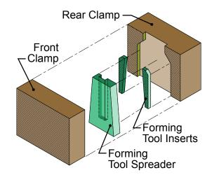
Figure 25. Exploded view of typical spreader assembly
