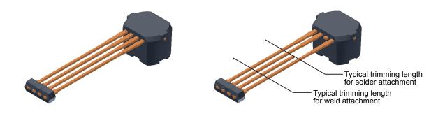
Figure 14. SG package (left) before trimming of pin 3, and (right) after trimming; note that it is not necessary to remove the package from the clamps, if the clamps are designed to also be used in the next step, bending by roller forming
