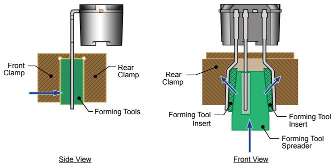
Figure 24. Clamping solution for pin trimming; bottom clamp forms an anvil on the bottom edge
