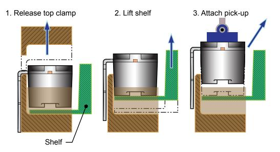
Figure 23. Integration of a shelf in the clamp fixture allows mechanical separation of the device from bottom clamp, allowing device extraction by a magnetic pick-up
