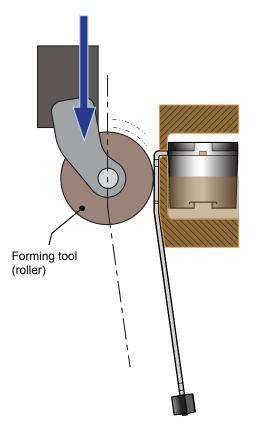
Figure 19. Roller forming with a bevel on the bottom clamp to accommodate pin spring-back
