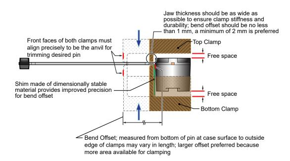
Figure 11. The bend offset can be set at any distance from the device body, because the clamps isolate the leadform operation forces from the case; as a good practice, ample free space should be left above and below the device body, to avoid incidental pressure that could disturb the internal wiring connections
