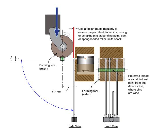
Figure 18. Side view (left), and front view (right) of roller forming; bottom clamp does not provide for pin spring-back after forming
