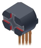
Figure 5. Coarse alignment features are provided for angular orientation in the final assembly module or carrier, but they should not be used in tight-tolerance automated operations for orientation because of tool wear against the abrasive case material.
