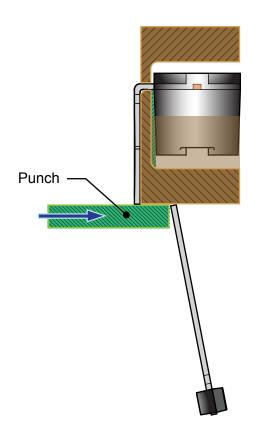
Figure 21. Clamping solution for pin trimming; bottom clamp forms an anvil on the bottom edge
