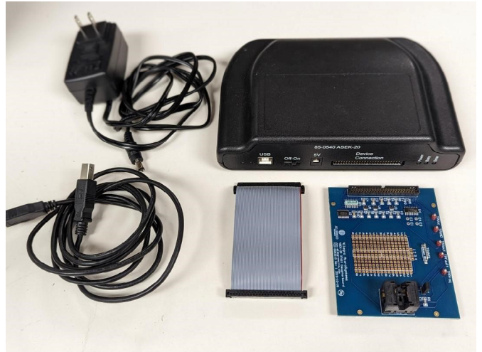
Figure 7: Connection between ASEK-20 and ACS37610 Daughterboard
