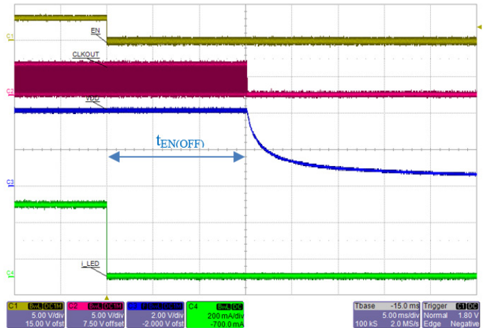
Figure 37: After EN = L for 32k clock cycles (~15 ms at 2.15 MHz), the IC completely shuts down so VDD (Blue) decays.
