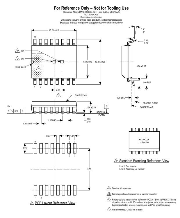
Figure 8: Package MA, 16-Pin SOICW
