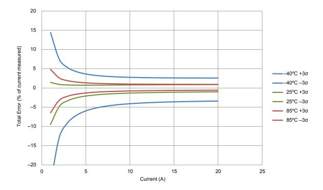
Figure 3: Predicted Total Error as a Function of Sensed Current for the ACS724KMATR-20AB
