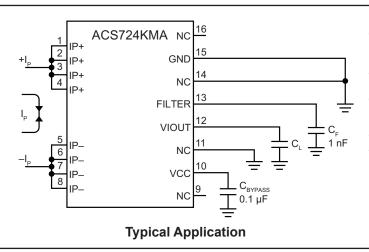
The ACS724KMA outputs an analog signal,  $V_{IOUT}$ , that changes proportionally with the bidirectional AC or DC primary sensed current,  $I_p$ , within the specified measurement range.
