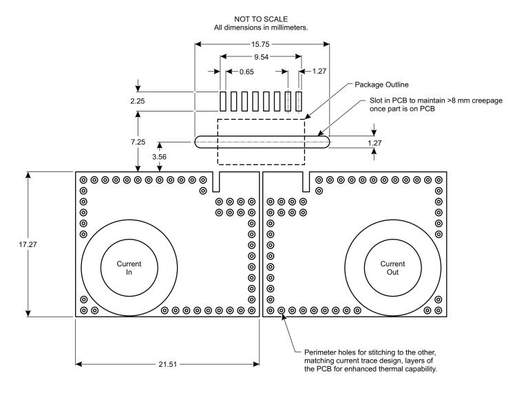
Figure 7: High-Isolation PCB Layout
