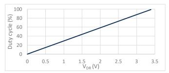
Figure 2: Relationship of External Voltage Input on VDR Pin and Dimming Duty Cycle.  $V_{DR}$  can be varied from 0 to 3.6 V.
