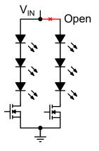
Figure 10: LED Open Protection
