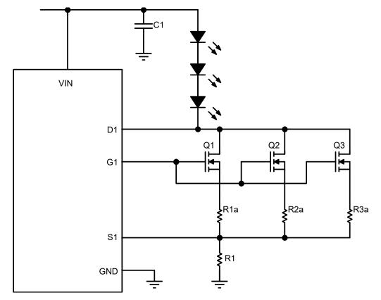
Parallel MOSFET Arrangement for High-Power Application
