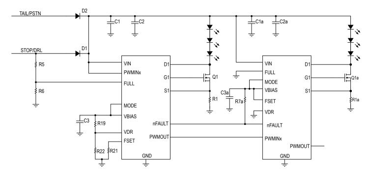
Figure 25: Master-Slave Operation with Internal PWM. Only one channel shown for simplicity.
