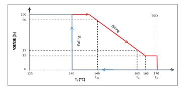
Figure 20: Output Current Foldback Based on Rising T<sub>J</sub>
