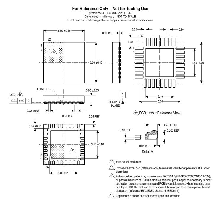
Figure 31: 32-Pin 5 mm × 5 mm QFN with exposed thermal pad and wettable flank (suffix ET)
