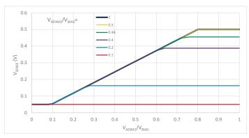
Figure 6: Combined Effect of ADIM1 and ADIM2 pin voltages on V<sub>SENSE</sub> for A80804
