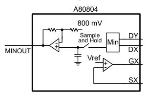
Figure 8: Block Diagram of MINOUT Block
