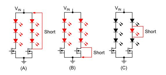
**Figure 14: Short-Circuit Protection**
