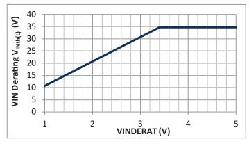
Figure 18: V<sub>INDERAT</sub> Voltage versus V<sub>IN</sub> Derating Threshold
