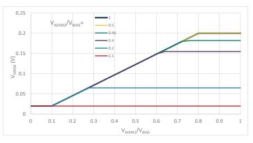
Figure 7: Combined Effect of ADIM1 and ADIM2 pin voltages on V<sub>SENSE</sub> for A80804-1
