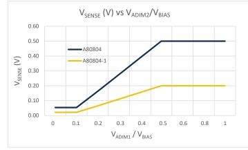
Figure 5: Effect of ADIM2 on V<sub>SENSE</sub>
