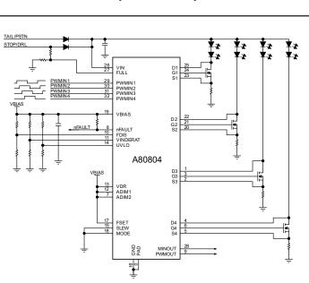
Figure 1: Typical Application Diagram with External PWM
