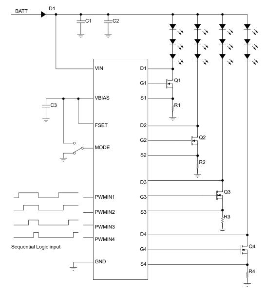
**Figure 27: Sequential LED driver** Each sequence is about 50-200 ms and off period could be up to 0.6 seconds. Faults will reset in each cycle as off period is > 20 ms.
