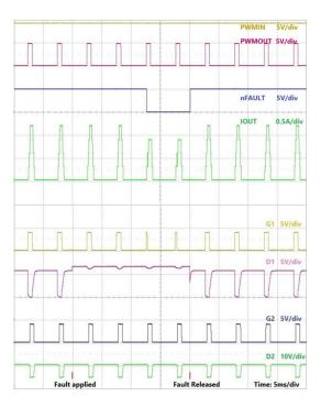
Figure 17: Drain Short to VIN Fault on D1 with Internal PWM Dimming. MODE = High (left), MODE = Low (right).
