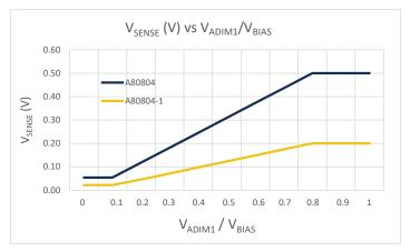
Figure 4: Effect of ADIM1 on V<sub>SENSE</sub>
