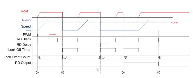
Figure 5: RD Timing Diagram (LOCKEVT = 0); lock condition while running
