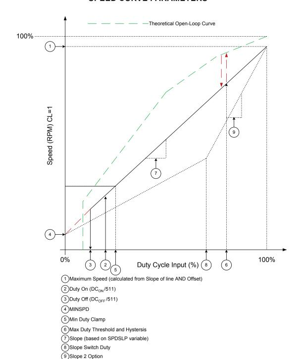
Figure 3: Speed Curve Parameters
