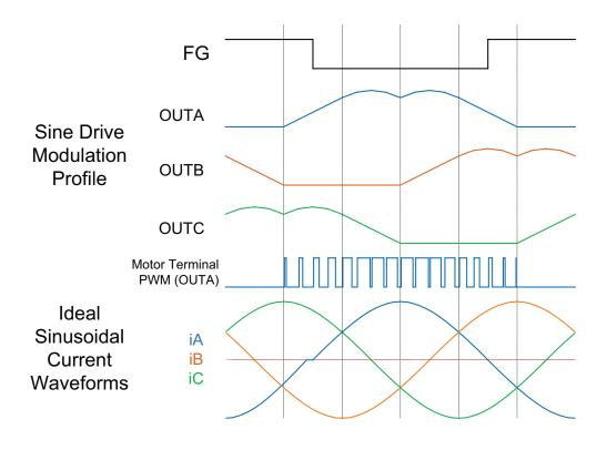
Figure 2: Sinusoidal Drive Sequence for DIR = HI
