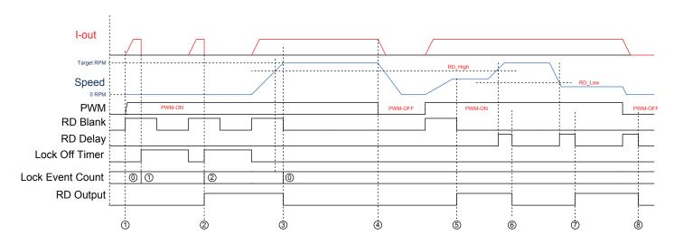
Figure 4: RD Timing Diagram (LOCKEVT = 0)
