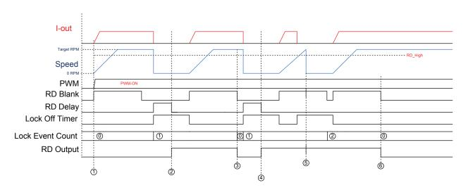
Figure 7: RD Timing Diagram (LOCKEVT = 1); lock condition while running
