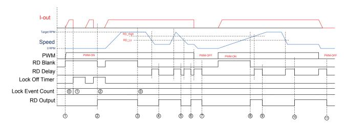
Figure 6: RD Timing Diagram (LOCKEVT = 1)
