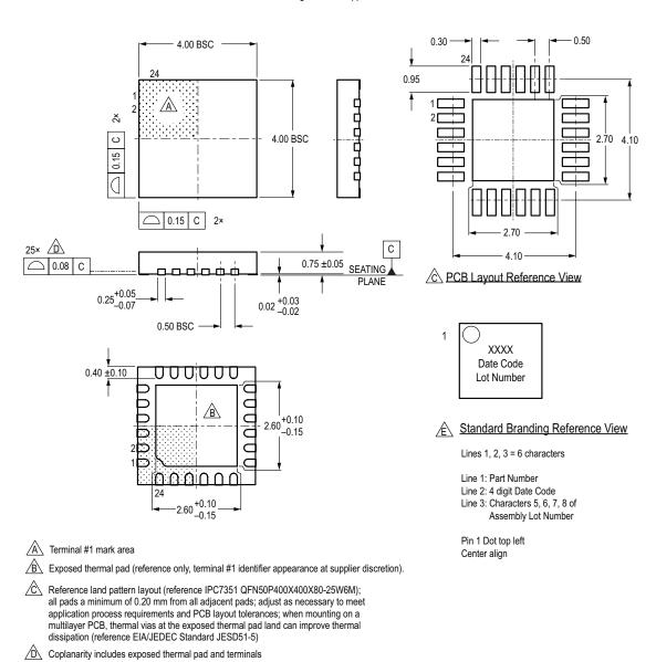
Figure 15: Package ES, 24-Contact QFN with Exposed Pad
