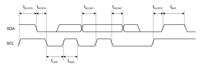
Figure 10: I<sup>2</sup>C-Compatible Timing Requirements
