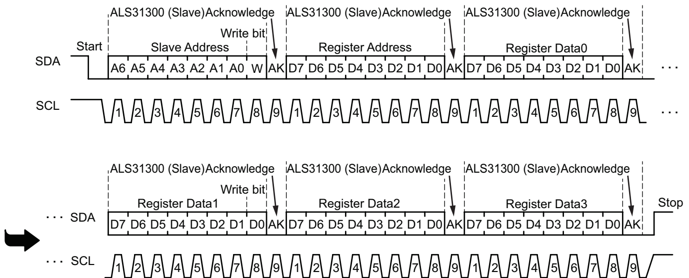
Figure 3: I 2 C Write Timing Diagram
