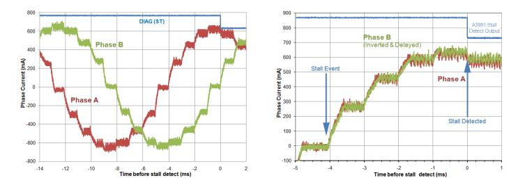
Figure 4. Typical behavior of bipolar stepper drive at a stall condition; (left) waveforms in normal phase, (right) waveforms adjusted for comparison
