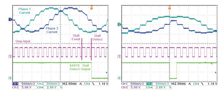
Figure 5. Typical hard stall behavior; (left) motor continuing to attempt to rotate in same direction, (right) motor reversing direction
